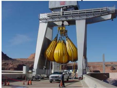
Crane testing at Glen Canyon Dam, 2005
