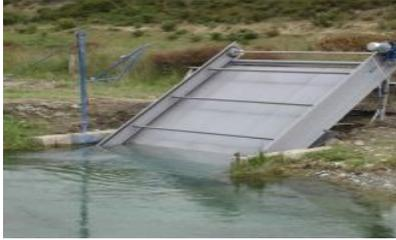
bank and removed by the farmer. The Aqwell didymo screen elements are sized to handle flows from 200 to 2000 liters a second. Screens range in cost from \$25,000 to \$50,000, depending on size. (*Excerpted from a Neal Wallace, Otago Daily Times article, September 19.*)
