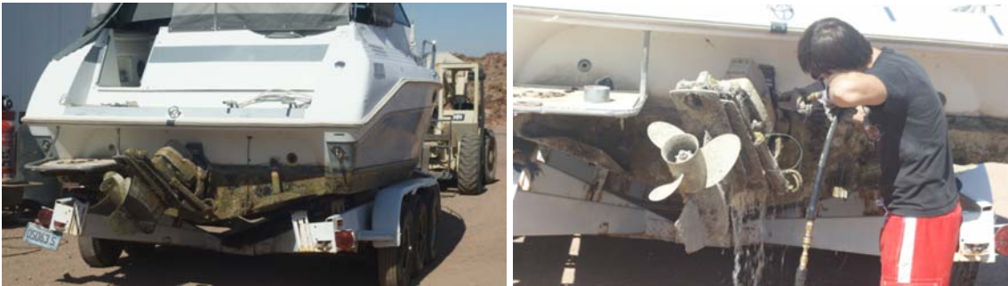
Figure 2. Field data validation on gimbal unit area with hot-water spray (140°F/5 seconds duration)
