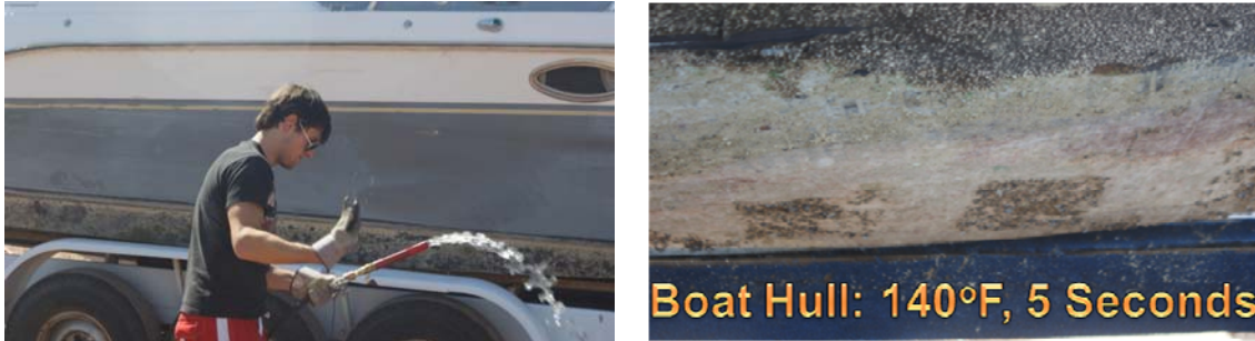
Figure 1. Field data validation on boat surface area with hot-water spray (140°F/5 seconds duration)
