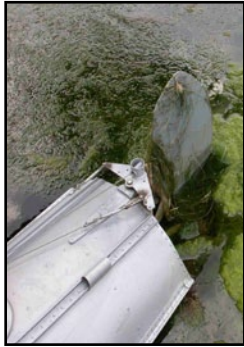
Fouled rudder - Lake Hood floatplane (USFWS)
